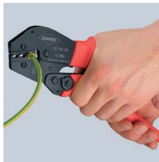
Third step: when greater hand force is required, such as e.g. when crimping insulated connectors 6 mm 2 , two-hand operation is possible by the longer handles
