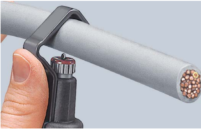
Setting the tool for circular cutting
