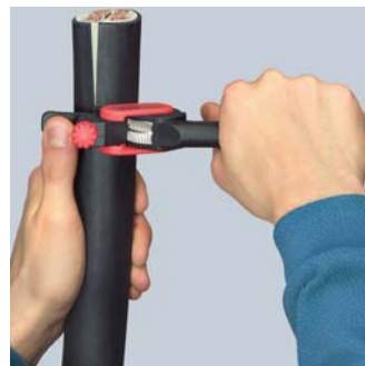
Turning the tool for circumferential cut
