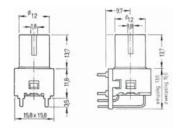
Key switch with plastic case and plastic key
