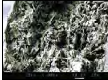
● Picture taken at 1,000x magnification using a SEM to demonstrate the fibrous nature of the FlexiCap™ termination that absorbs increased levels of mechanical stress.
