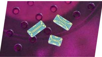
DLI's surface mount directional coupler series span the frequency spectrum of C, X and Ku bands. Both 10dB and 20dB coupling values are available within each frequency band both with a common footprint for maximum flexibility. These couplers incorporate DLI's low loss high permittivity ceramics which provide small size and temperature stability. These couplers offer a turnkey surface mount solution for high frequency power monitoring. Custom solutions are also available.
