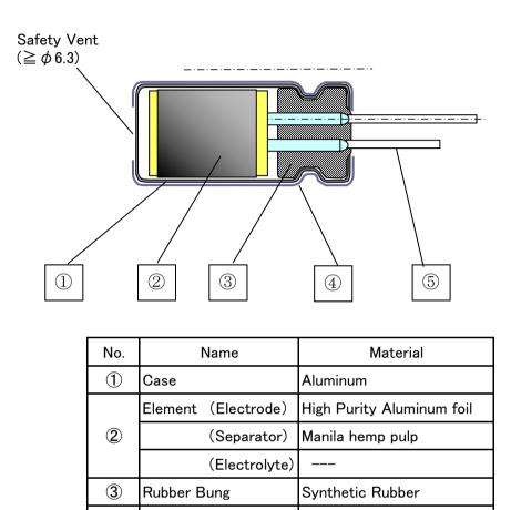
5 Lead Wire Tin plated Steel Wire
