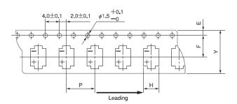
Fig. 1-2 Carrier tape  $\phi$ D≥12.5
