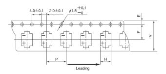
Fig. 1-2 Carrier tape  $\Phi D \ge 12.5$
