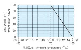
在环境温度70℃以上使用时,应按照左图负荷减轻特性曲线,减小额定功率。 For resistors operated at an ambient temperature of 70℃ or above, a power rating shall be derated in accordance with the left derating curve.
