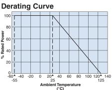
For resistors operated at an ambient temperature of  $25^{\circ}$ C or above, a power rating shall be derated in accordance with the above derating curve.
