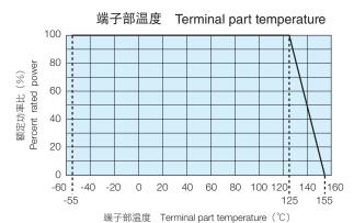
超过上述端子部温度使用时,请根据负荷减轻特性曲线减小额定功率后使用。 ※ 关于使用方法,请参照卷首的"端子部温度负荷减轻特性曲线的说明"。 For resistors operated terminal part temperature of described for each size or above, a power rating shall be derated in accordance with derating curve. \*Please refer to "Introduction of the derating curves based on the terminal part temperature" on the beginning of our catalog before use.
