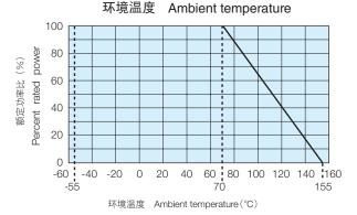
在环境温度70℃以上使用时,应按照上图负荷减轻特性曲线,减小额定功率。 For resistors operated at an ambient temperature of 70°C or above, a power rating shall be derated in accordance with the above derating curve.
