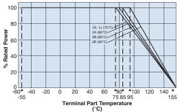
For resistors operated terminal part temperature of described for each size or above, a power rating shall be derated in accordance with derating curve. Please refer to "Introduction of the derating curves based on the terminal part temperature" in the beginning of our catalog before use.
