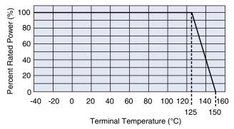
For resistors operated at a terminal temperature of 125°C or above, a power rating shall be derated in accordance with the above derating curve.
