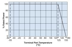
For resistors operated terminal temperature of described for each size or above, a power rating shall be derated in accordance with the derating curve. Please refer to "Introduction of the derating curve based on the terminal part temperature" in the beginning of our catalog before use.
