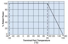
For resistors operated terminal temperature of described for each size or above, a power rating shall be derated in accordance with the derating curve above. Please refer to "Introduction of the derating curve based on the terminal part temperature" in the beginning of our catalog before use.
