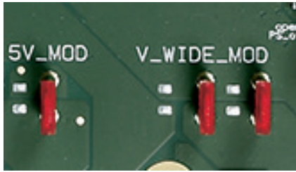
Figure 19: Jumpers 5V_MOD and V_WIDE_MOD
