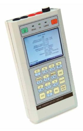
The KE-TDR20 has been designed for quick and accurate fault location and qualification of balanced telecommunication cables. The various measuring modes provide accurate location of discontinuities and errors like open circuits, wet sections, loose contacts etc.
