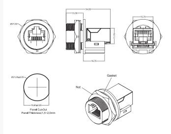
\*Kit includes jack, nut, and gasket Recommended Nut Torque: 12 Kgf-cm
