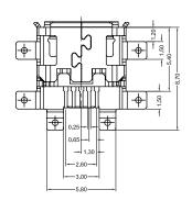
Rated Voltage: 30V AC (RMS) Current Rating: 1A Dielectric Withstanding Voltage: 100V AC
