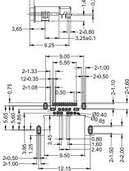
Recommended PCB Layout Suggested PCB Thickness: 0.60 mm (Top View)
