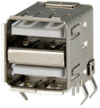
KUSBX Right Angle PCB Mount A&B Type
