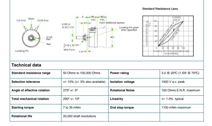
High quality, general purpose wirewound panel control of robust and reliable construction. Phenolic body moulding; nickel silver contact; nickel plated brass spindle and bush electro-tin plated brass termination tags.
