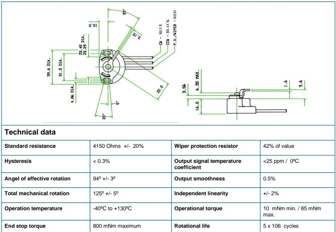
Conductive polymer potentiometer for automotive and other similar demanding applications. A high performance cost effective potentiometer, with long endurance life and protection from engine compartment environment. Termination via 280 mm long flying leads.
