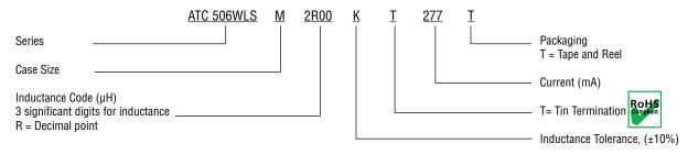
The above part number refers to a 506WLS Series, Case Size M, 2.00 µH inductor, K tolerance (±10%, typ.), with Tin Termination (T), 277 mA, tape and reel packaging.
