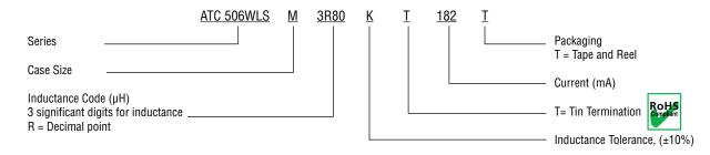
The above part number refers to a 506WLS Series, Case Size M, 3.80 µH inductor, K tolerance (±10%, typ.), with Tin Termination (T), 182 mA, tape and reel packaging.
