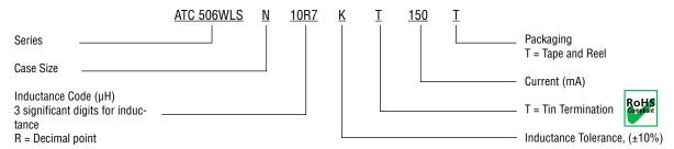
The above part number refers to a 506WLS Series, Case Size N, 10. 7 µH inductor, K tolerance (±10%, typ.), with Tin Termination (T), 150 mA, tape and reel packaging.
