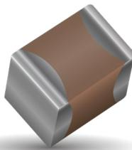
The X7R dielectric is the most popular of the intermediate EIA class II materials due to its relative temperature stability. While the capacitance change is non-linear, temperature variation is within  $\pm 15\%$  from  $-55^\circ\text{C}$  to  $+125^\circ\text{C}$ .
