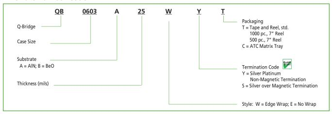
The above part number refers to a Q-Bridge, (EIA case size 0603), Aluminum Nitride (AIN) substrate, Thickness 25 mils., Style W, Y Termination (Silver Platinum Non-Magnetic Termination), with Tape and Reel Packaging.
