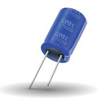
The new series of cylindrical electrochemical double-layer capacitors offers excellent pulse power handling characteristics based on the combination of very high capacitance and very low ESR. Used by themselves or in conjunction with primary or secondary batteries, they provide extended back up time, longer battery life, and provide instantaneous power pulses as needed. Offers great solutions to Hold Up, Energy Harvesting, and Pulse Power Applications.
