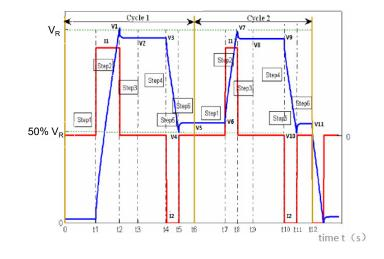
Note: I<sub>1</sub> = I<sub>2</sub> = 75mA/F, the rated capacitance in the chart means discharge capacitance, and DC ESR (ESR<sub>DC</sub>) means discharge DC resistance.
