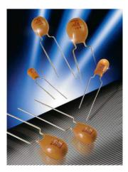
TAP is a professional grade device manufactured with a flame retardant coating and featuring low leakage current and impedance, very small physical sizes and exceptional temperature stability. It is designed and conditioned to operate to +125°C (see page 282 for voltage derating above 85°C) and is available loose or taped and reeled for auto insertion. The 15 case sizes with wide capacitance and working voltage ranges means the TAP can accommodate almost any application.
