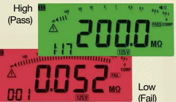
Easy to identify low or high resistance by LCD backlight color.
