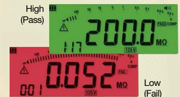
Easy to identify low or high resistance by LCD backlight color.
