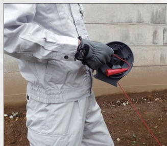
Innovative Cable reel with wire guide system to facilitate rewinding
