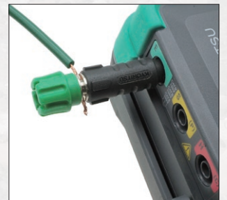
Adapter to enable use of other test leads
