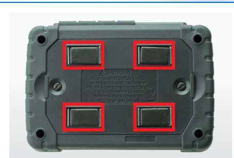
Strong magnets help to fix KEW5050 to the metal distribution board.
