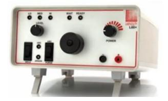
The Thermocouple Welder is a compact, simple-touse instrument designed for thermocouple and fine wire welding
