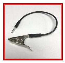
Impact welding is the term used for welding wires to a conductive metal surface. This process is common when thermocouples are required to be welded to a test piece/structure or similar application.
