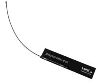
The Revie Flex (EFF692SA3S) is a flexible PCB antenna for use in LTE CAT M1 and NB-IoT devices. The antenna is optimized for use when mounted to plastic via the supplied adhesive backing. This antenna operates within 698 - 875 MHz and 1710 – 2500 MHz with excellent radiation performance. The high efficiency ensures reliable connection in a variety of integration environments.
