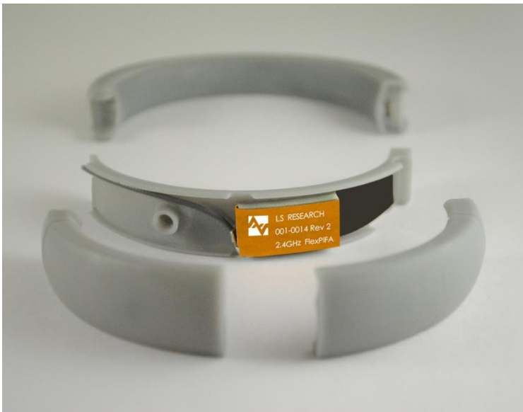
Figure 27: FlexPIFA integrated into bracelet
