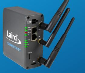
The Sentrius™ IG60 brings all of Laird Connectivity's industrial wireless and IoT capabilities into one unique solution. Based on Laird Connectivity's 60-series and BL654, capture data from legacy serial (RS-232, 422, 485) industrial devices or Bluetooth 5 sensors, add cloud-managed edge intelligence, and send to the cloud with 802.11ac Wi-Fi and global LTE Cat 1 wireless connectivity.
