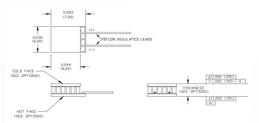
Ceramic Material 96% Alumina Ceramics Solder Construction: 271°C, Proprietary
