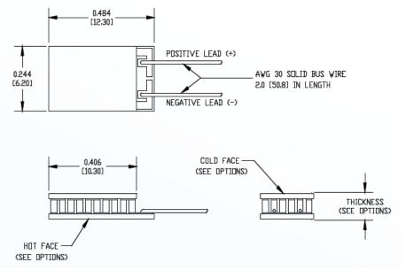
Ceramic Material: 96% Alumina Ceramics Solder Construction: 232°C SnSb
