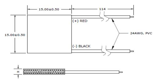
Ceramic Material: Alumina(Al2O3) Solder Construction: 138°C BiSn
