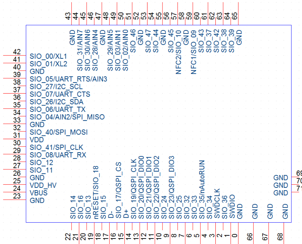
Figure 3: BL654 module pin-out (top view). Outer row pads (long red line) and inner row pads (short red line) shown.
