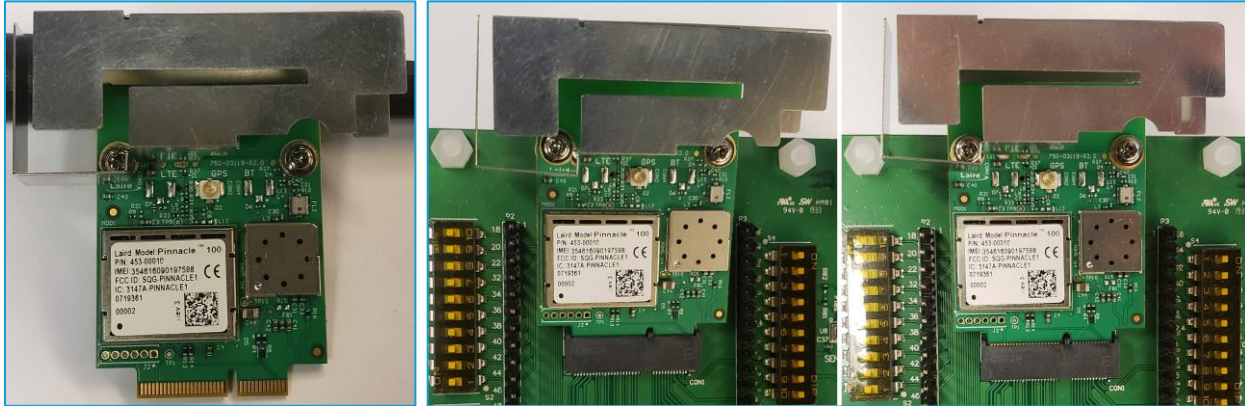
Figure 7: Attaching a 453-00010 Pinnacle™ 100 modem to a DVK
