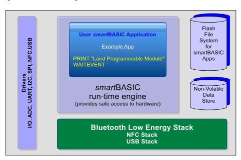
Figure 2: Functional HW and SW block diagram for BL654PA BLE module
