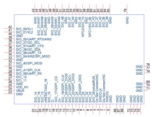
Figure 3: BL654PA module pin-out (top view). Outer row pads (long red line) and inner row pads (short red line) shown.
