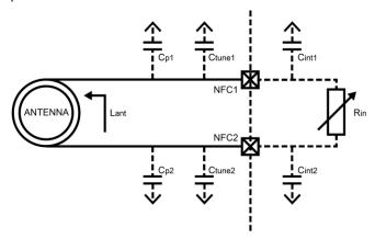
Figure 5: NFC antenna coil tuning capacitors
