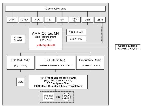
Figure 1: BL654PA block diagram
