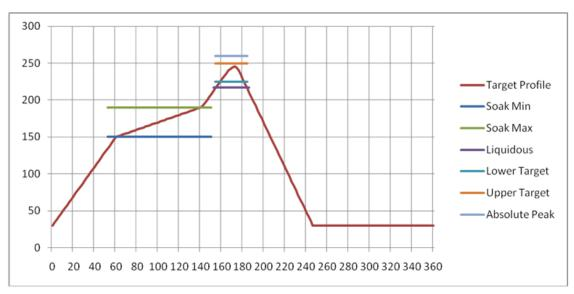
Figure 17: Recommended reflow temperature
