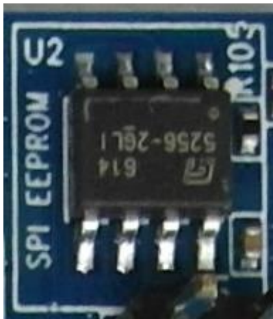
Figure 17: SPI EEPROM schematic and PCB
