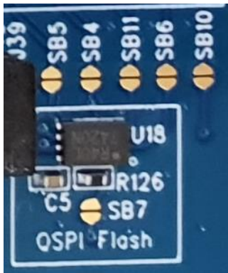
Figure 20: Optional external serial SPI flash IC (U18) schematic and PCB
