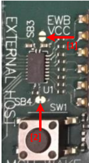
Figure 7: External HOST interface schematic and location of solder bridge modifications
