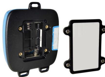
Figure 2: Back side of the Sentrius™ RS1xx sensor
