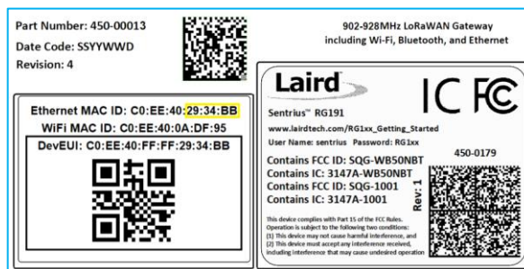
Figure 4: Bottom label (Standard GW – Left, AS923 & AU915 Region Supported/Latest Version – Right)– last three bytes of the Ethernet MAC address highlighted
