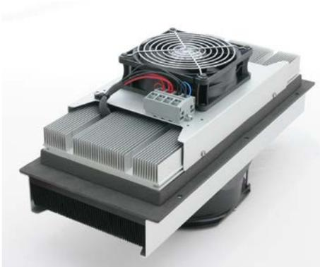
The AA Outdoor Cooler Series is an air-to-air thermoelectric assembly (TEA) that uses impingement flow to transfer heat. It offers dependable, compact performance by cooling objects via convection. Heat is absorbed and dissipated thru high density heat exchangers equipped with air ducted shrouds and brand name fans. The heat pumping action occurs from custom designed thermoelectric modules that achieve a high coefficient of performance (COP) to minimize power consumption.
