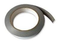
Laird DT03B double sides conductive fabric tape is constructed of metallized fabric with pressure sensitive adhesives on both sides. With the unique technology and design, the z-axis resistance of DT03B is less than 0.03ohm and stable even under very small area. It also provides good adhesion and EMI shielding performance.
